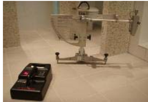
Slip Testing Anti Slip Treatment
