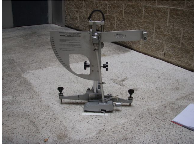
Slip testing a sample of a non slip treatment
